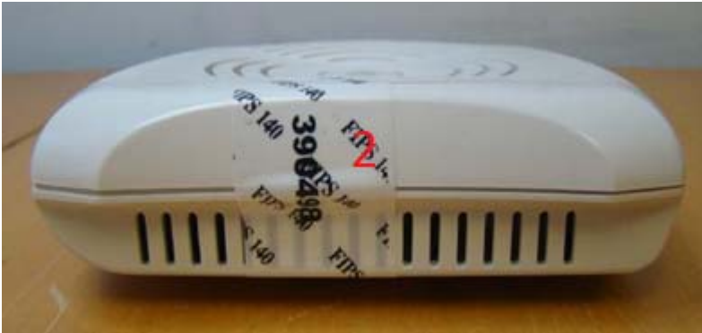
Figure 7 - Aruba AP-93 TEL placement left view
